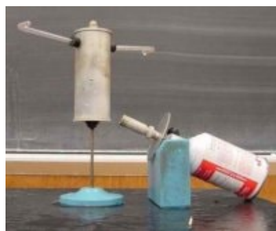
Heron's Engine Blowtorch ( Creative Commons [2] )
