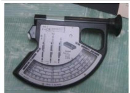
A clinometer based upon same principles as the protractor device (Public Domain)
